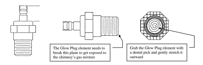
clears the plane of the end of the glow plug (see drawing below)
